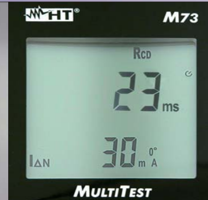
Tripping time measure performed on a RCD type AC (M73 only)
