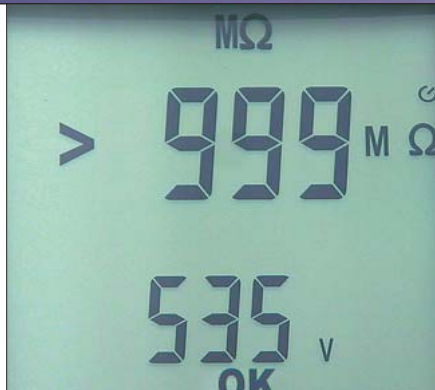
Insulation measure with 500VDC test voltage (M72 only)
