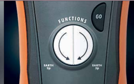
Electronic function selector of M71
