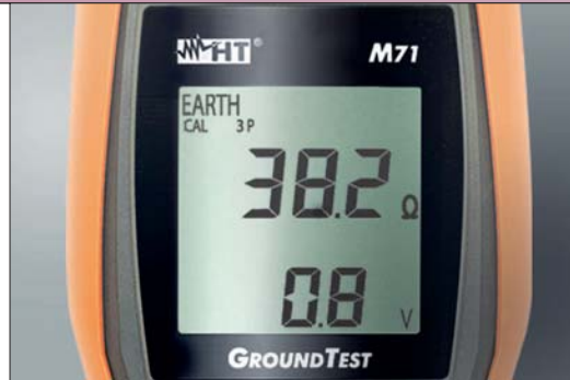
Earth measure (3-wire method)
