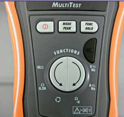
Electronic function selector of M72
