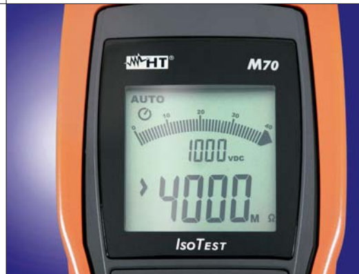
Insulation measure (1000VDC)
